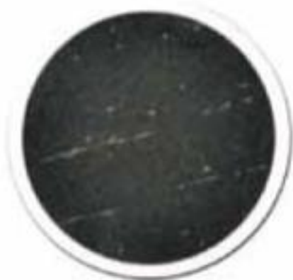
No retrofit system Uncontrolled Diesel Exhaust (Level 1)
