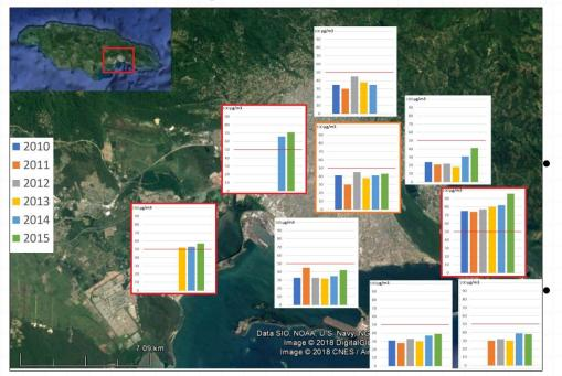
Map showing trends in annual average concentrations for  $PM_{10}$  in KMA. Red line indicates Jamaican Standard for ambient  $PM_{10}$ . Out-of-compliance stations are highlighted with a red line border. The stations with saturation conditions (close to being out of compliance) are highlighted with an orange line border.
